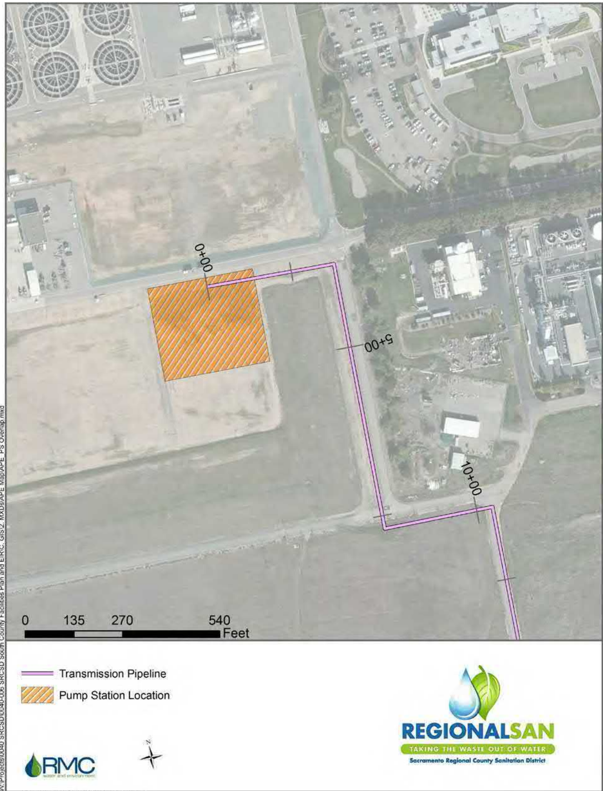
Figure 2-3: Proposed Pump Station Site
