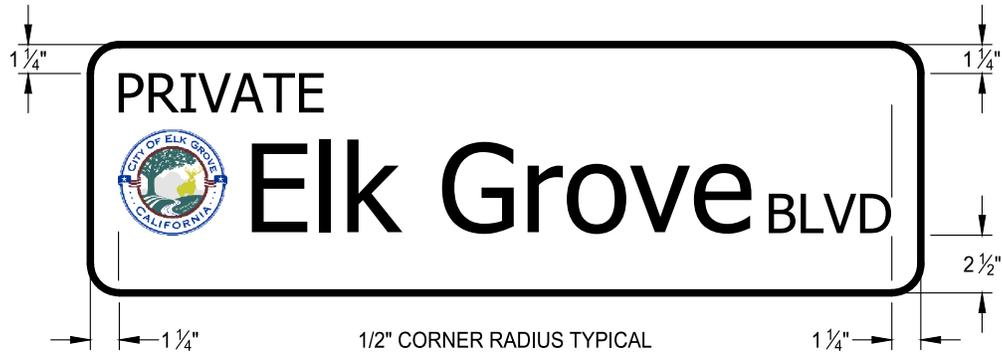
**SIGN BLANKS:** ALL STREET NAME SIGNS SHALL BE 10 INCHES IN HEIGHT, A MINIMUM OF 30 INCHES IN LENGTH AND A MAXIMUM OF 42 INCHES IN LENGTH. SIGN BLANKS SHALL BE 0.080 INCH THICK, ASTM B209 ALLOY 6061-T6, FLAT ALUMINUM FOR CANTILEVER MOUNTED SIGNS AND SHALL BE 0.125 INCH THICK, ASTM ALLOY 6061-T6, FLAT ALUMINUM FOR CENTER MOUNTED SIGNS.
