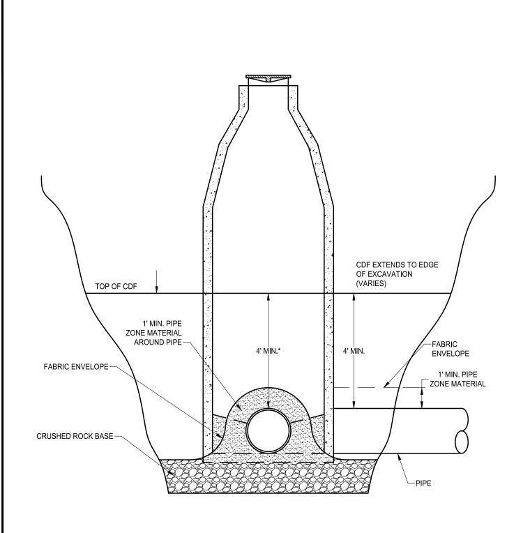
\*OR THE BASE OF CONE, WHICHEVER IS LESS. FLATTOP MANHOLES, CDF TO BE PLACED NO HIGHER THAN SUBGRADE.
