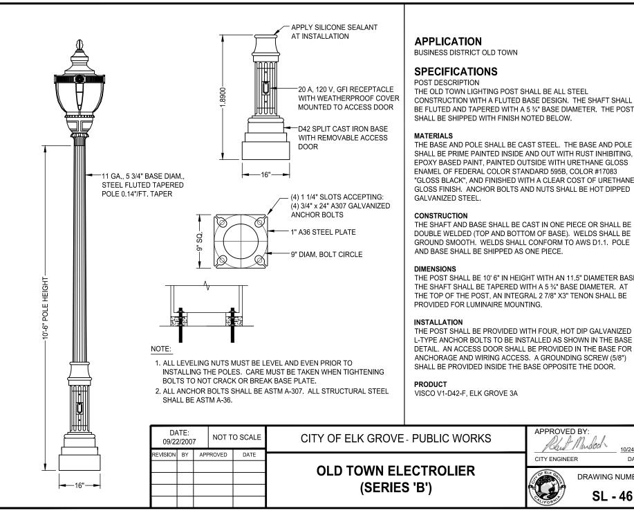
THE POST SHALL BE PROVIDED WITH FOUR. HOT DIP GALVANIZED L-TYPE ANCHOR BOLTS TO BE INSTALLED AS SHOWN IN THE BASE DETAIL. AN ACCESS DOOR SHALL BE PROVIDED IN THE BASE FOR ANCHORAGE AND WIRING ACCESS. A GROUNDING SCREW (5/8") SHALL BE PROVIDED INSIDE THE BASE OPPOSITE THE DOOR.
