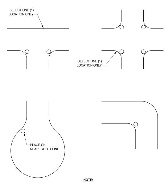
IN ACCORDANCE WITH STREET CLASSIFICATIONS, ALL ARE SERIES 'A' OR SERIES 'B' STREET LIGHTS WITH ANSI TYPE III LIGHT DISTRIBUTIONS PATTERN. SEE STANDARD DRAWINGS SL-2 AND SL-24
