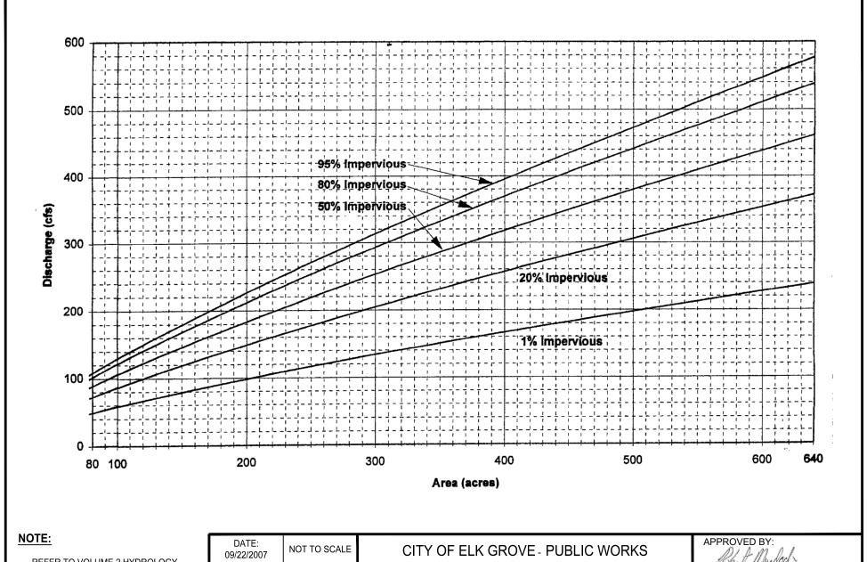
REFER TO VOLUME 2 HYDROLOGY STANDARDS OF THE CITY/COUNTY DRAINAGE MANUAL FOR ASSUMPTIONS MADE IN DERIVING THIS FIGURE.
