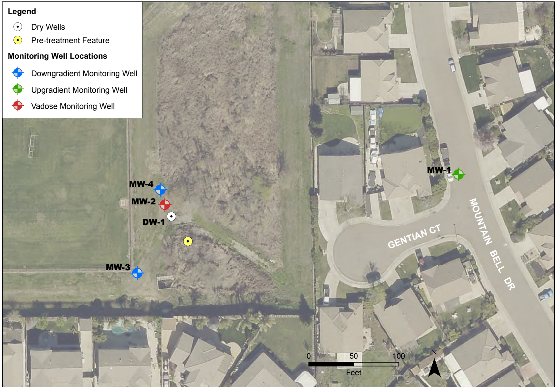
Figure 3-1 Location of Dry Well and Monitoring Well Network Site 1: Strawberry Creek Water Quality Basin
