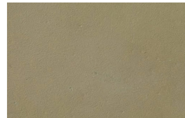
Example: 5447 Mesa Buff Concrete Color with Medium Broom Finish*
