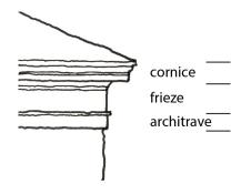
Fascia. A frieze or band running horizontally and situated vertically under a roof edge, often forming the outer surface of a cornice.
