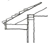
Bracket. An ornamental support, usually of wood or metal, which appears where the roof or balcony edge meets the exterior wall of the building.
