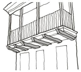
Balustrade. A railing consisting of a row of balusters, or small vertical posts, supporting a rail.
