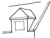
**Dormer, hipped-through-cornice.** A partially nested dormer with a hipped roof.
