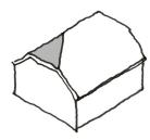
Roof, front-gabled. A roof comprising a single pitched element with front- and rear-facing gables.
