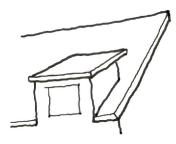
**Eave.** The lower edge of the portion of roof that overhangs the walls of a building.
