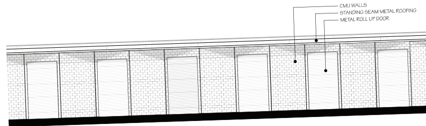
TYPICAL RV STORAGE BUILDING LAYOUT SCALE: 1/8" = 1'-0"
