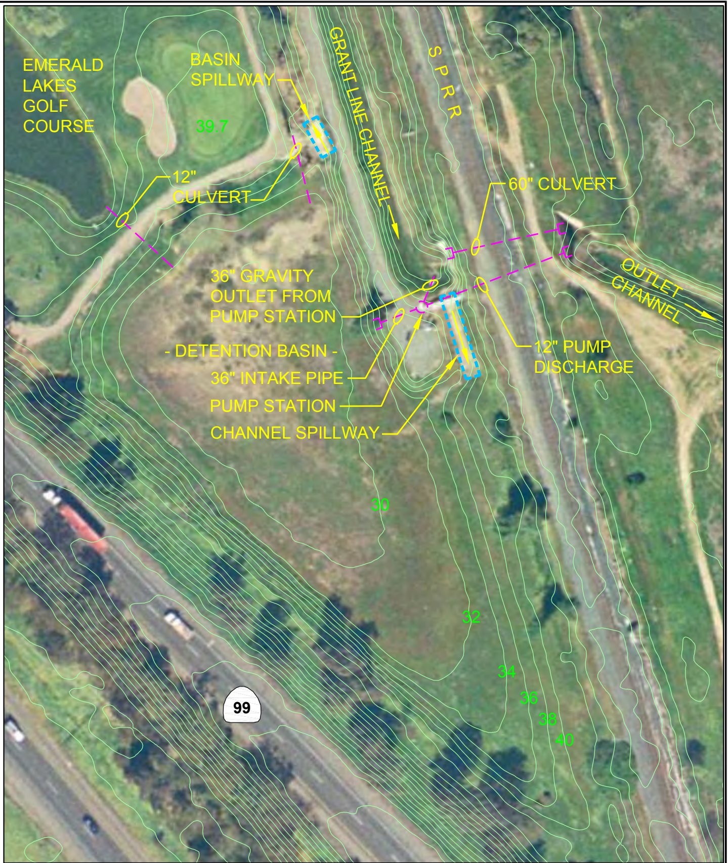
Figure 16-3 City of Elk Grove Storm Drainage Master Plan Volume II GRANT LINE CHANNEL EXISTING DETENTION BASIN & PUMP STATION
