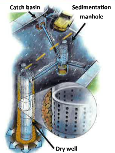
Figure 2. Schematic of typical city UIC system in Portland. Source: Portland Bureau of Environmental Services
