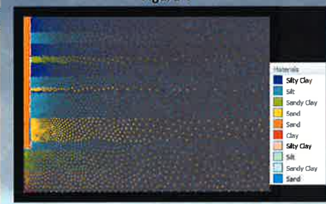
Figures 2 and 3. Lithologic cross-sections created using borehole data taken during monitoring well and drywell construction. Figures 4 and 5. Axisymmetrical HYDRUS 2D domains for SCDB and CY respectively (SCDB domain is 17 m by 24 m, and CY domain is 23 m by 24 m) created to represent the vadose zone materials portrayed in the cross-sections.
