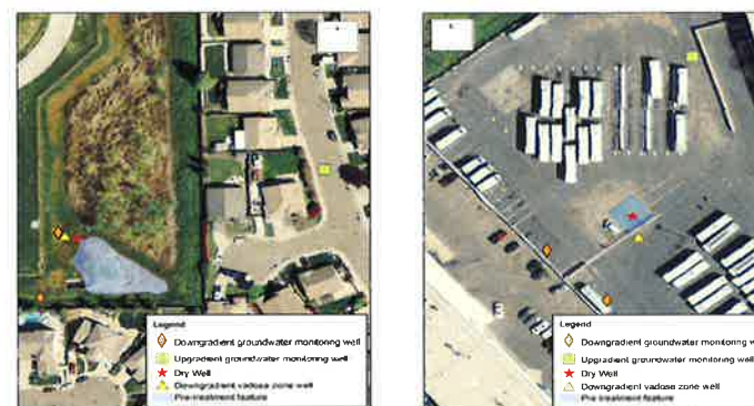
Figures 4a and b. Aerial photographs of the two study sites. The left panel is the Strawberry Creek site; the right panel is the City's Corporation Yard. Location of monitoring wells, dry well, and the vegetated pre-treatment features are shown.
