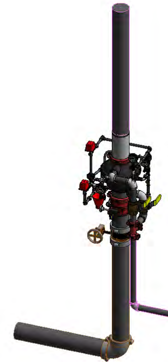
FIGURE 2: TYPICAL DRY-PIPE VALVE ASSEMBLY
