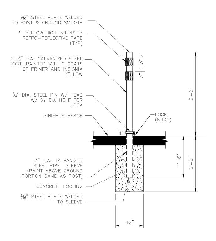
NOTE: DRILL A  $^{13}\!\!/_{6}$ " DIA HOLE THRU BOTH THE POST AND SLEEVE FOR PIN PLACEMENT
