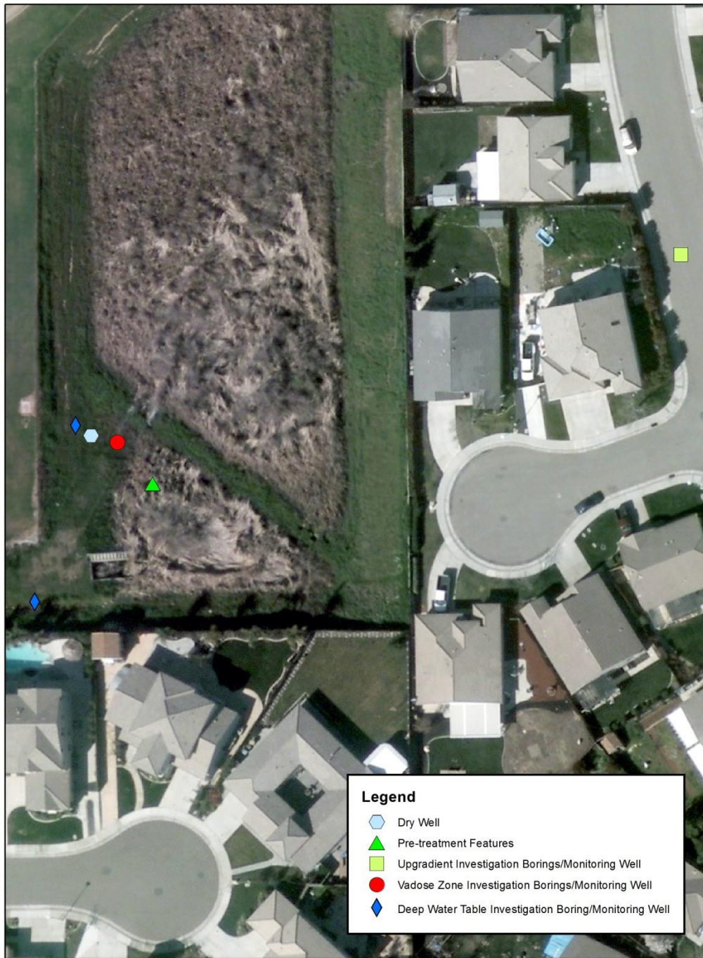
Exhibit 5. Diagram of Location of Dry Well and Monitoring Well Network at the Site 1: Residential Site -I Strawberry Creek Water Quality Basin
