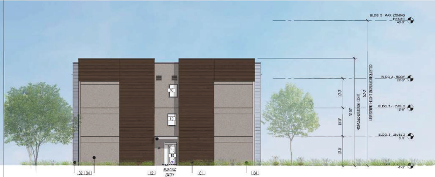
3 BLDG. B - EAST ELEVATION 18' x 14'
