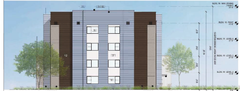
3 BLDG. J - EAST ELEVATION 1/8" = 1'-0"
